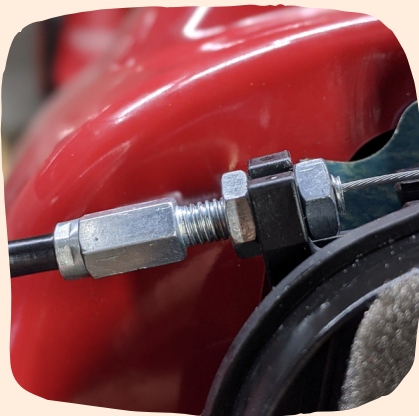
Figure 6: Jam nuts in the "forward" position
