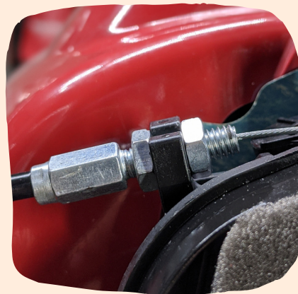
Figure 7: Jam nuts in the "backwards" position
